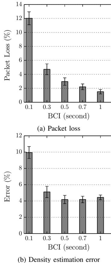
Fig. 2: Packet loss and density estimation error with default parameter settings
