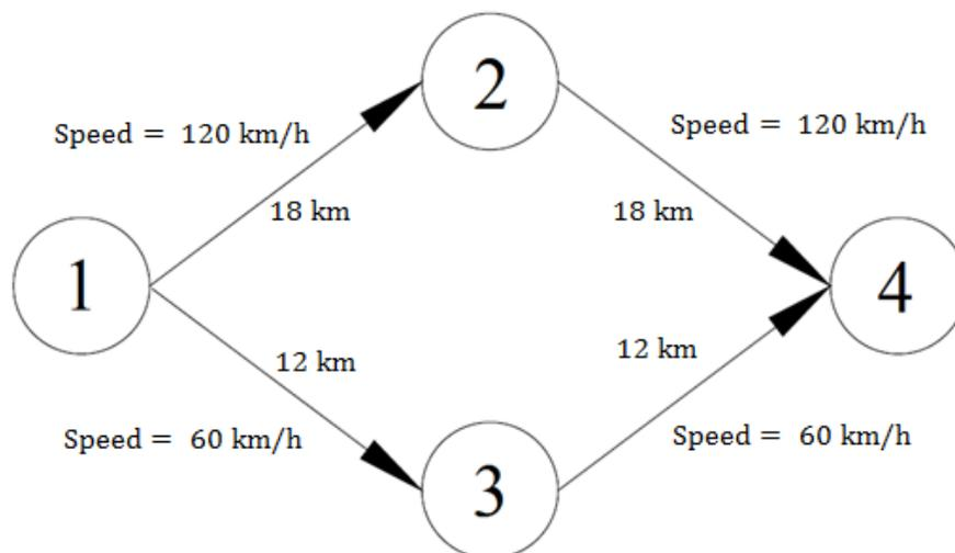
**FIGURE 1 Demonstration network with link lengths and free flow speeds**
