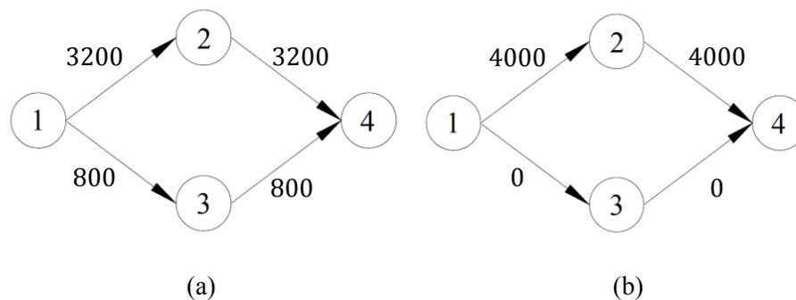
**FIGURE 2 Paradox Demonstration: (a) Link flows before the CS is built and (b) after the CS is built at node 2**
