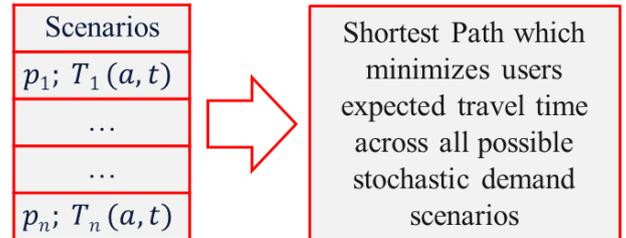
**Figure 1: Scenario-based Stochastic Time-Dependent Shortest Path.**  $p_i$  is the probability and  $T_i(a, t)$  is the travel time on arc  $a$  at departure time  $t$  in the scenario  $i$ .
