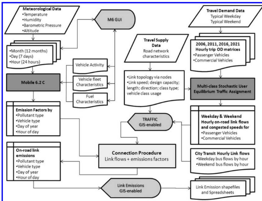
1 Modeling framework for estimating on-road link emissions with Mobile 6-2C
