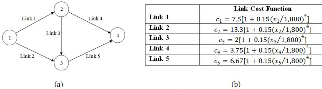
Figure 2: (a) Sample Network (b) Link Costs associated with the network
