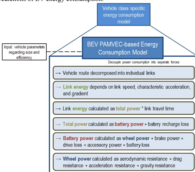
**FIGURE 3 Summary of how energy consumption is calculated for BEVs**
