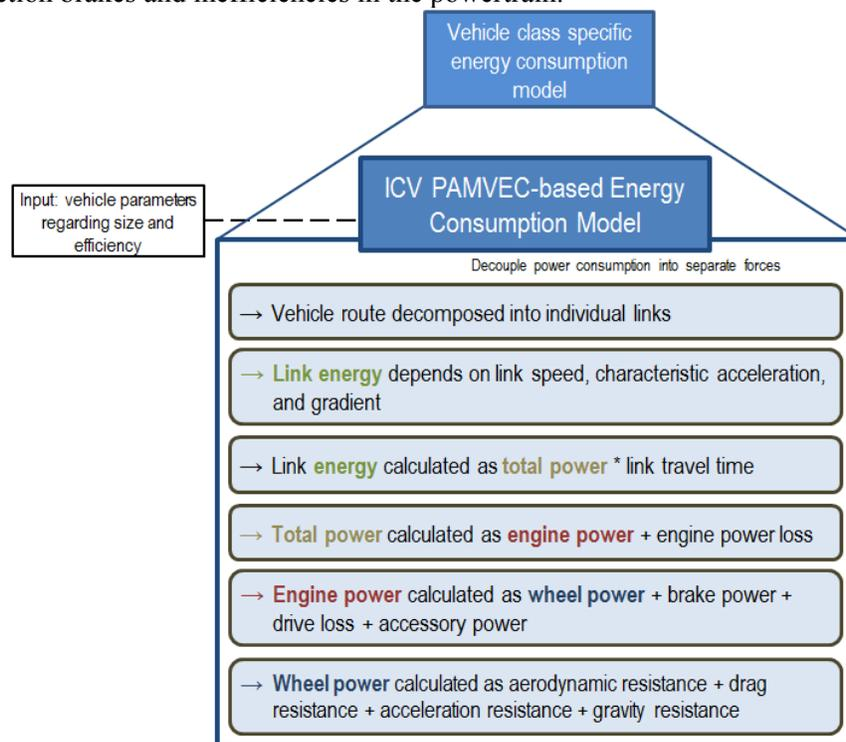
**FIGURE 2 Summary of how energy consumption is calculated for ICVs**
