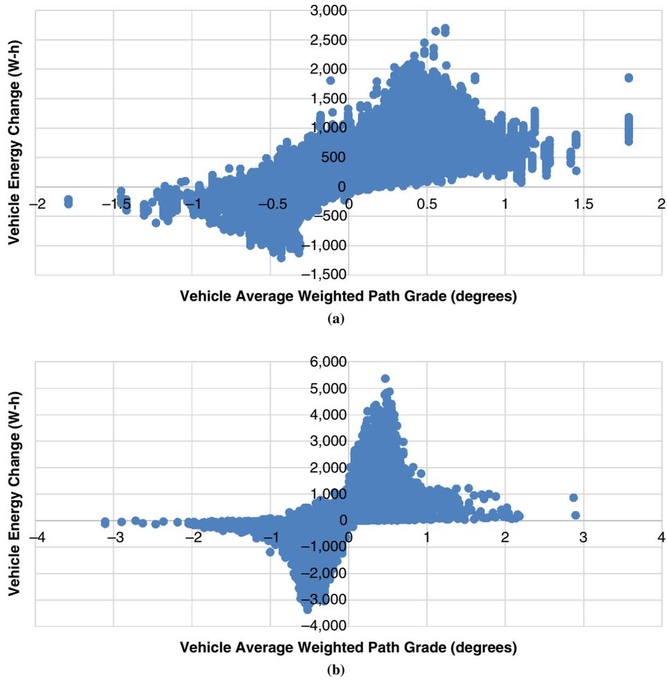
FIGURE 2 Energy change for individual vehicles because of inclusion of impact of link grade for (a) downtown Austin and (b) Nicosia networks.
