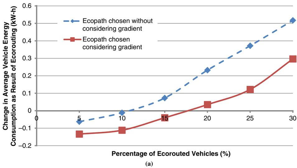
FIGURE 3 Change in energy consumption per vehicle for drivers using ecorouting by percentage: (a) downtown Austin network.
