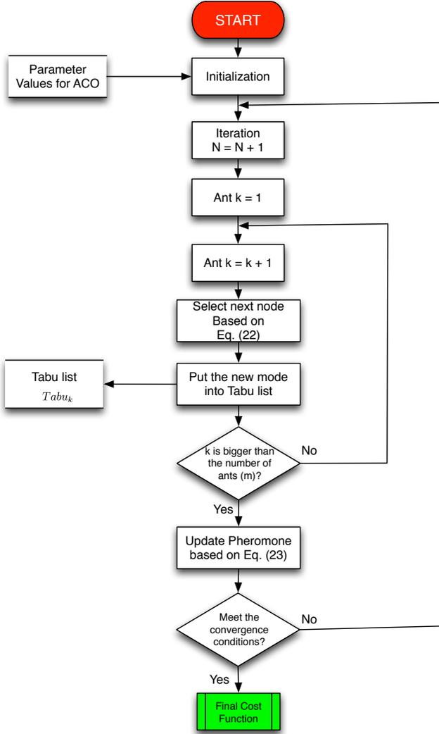
Fig. 2. Workflow of ACO-based Scheduler
