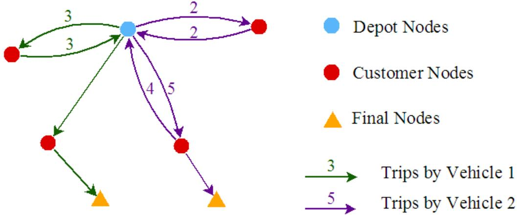
Figure. 1 – An example of a solution for the S-RMCDP with two vehicles; the number besides an arc indicates if this trip is repeated more than once.
