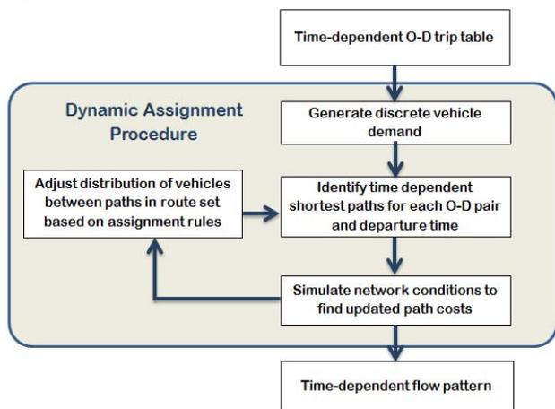
Fig. 2. Overview of the DTA Procedure
