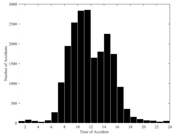
Figure 3 – Number of construction accidents for each time slot
